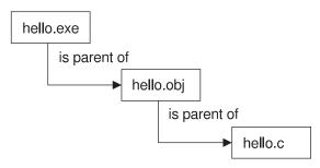
Figure 45. The build tree for the hello application
